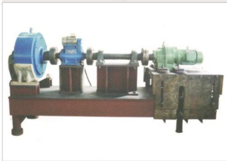
转矩转速功率测量仪 Measure instrument for torque, rotation rate and power
